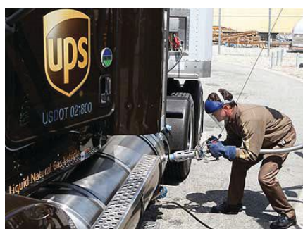
Liquid natural gas (LNG) UPS fleet vehicle being fueled. (Photo courtesy of UPS)
